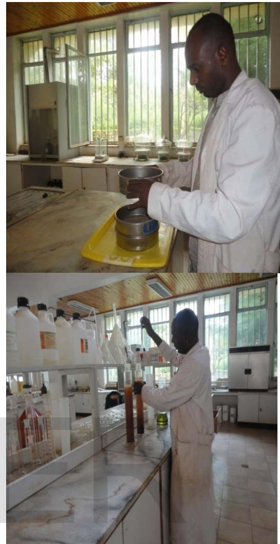
Figure 4.5: Soil Laboratory for Grain Size analysis (Wet-sieve and Hydrometer) Source: Wolaita Soddo Soil Laboratory Work on July, 2014
